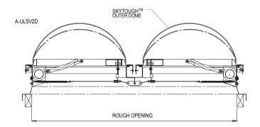
Non Listed Standard Smoke Vent Model No. Example: 4896-S-SV-DD-CM-ST-MF-OR-370° 4896 Steel frame Smoke Vent Double Dome Curb Mounted SkyTough-Mill Finish- Outside Release Fusable Link 370° Degrees
