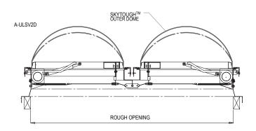
Non Listed Standard Smoke Vent Model No. Example: 4896-S-SV-DD-CM-ST-MF-OR-370° 4896 Steel frame Smoke Vent Double Dome Curb Mounted SkyTough-Mill Finish- Outside Release Fusable Link 370° Degrees
